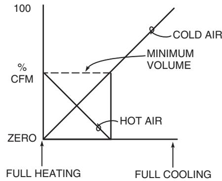
cold air volume is reduced as the cooling load drops until a minimum cfm is reached. After that point, heating and cooling are blended.
