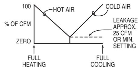
As the Therma-Fuser diffusers reduce cold air flow, the master zone responds to its static pressure controller positioning the cold air valve. When the master zone changes to heating, the cold valve is fully closed and the hot air valve modulates to supply Therma-Fuser subzone needs. A field adjustable minimum flow adjustment may be provided for the Therma-Fuser diffusers, but the master zone box supplies only hot air or cold air at one time.
