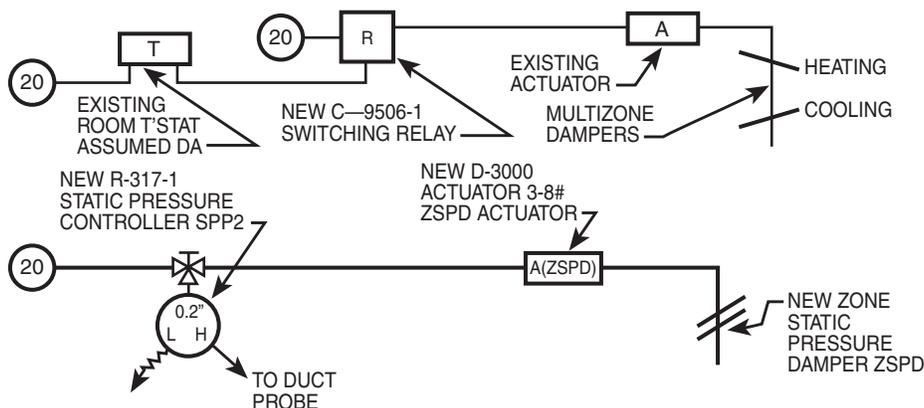
balancing dampers may be used for static pressure control.
