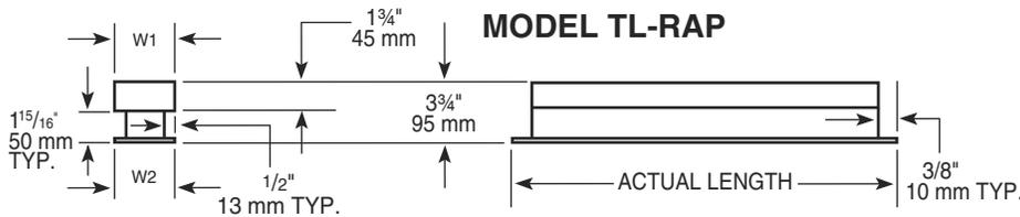
Note: Dimensions inches  $\pm$  1/16 millimeters  $\pm$  1.6 mm
